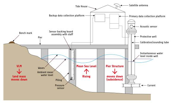
Figure 7: Typical modern tide gauge installation with components which contribute to measured Relative Sea Level rise (RSL).
